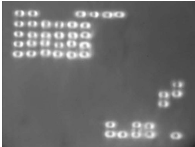
Fig. 7. Microscopy image of the time-shared optical trapping of 42 beads using AODs. This image demonstrates the smallest game of Tetris ever played. The corresponding video can be found online at http://www.nat.vu.nl/compl/dualdna/tetris .
