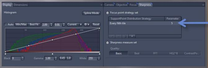
16. Under Sharpness, change the number in Parameter to 2 for small sections and 5 for larger sections (focusing will be performed every 2<sup>nd</sup>/5<sup>th</sup> tile).
