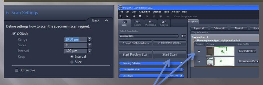
21. Press 'Finish'. These changes are local and they will be applied only to the slide next to the modified 'Scan Profile'. Press 'Start Scan'. See next page for applying these changes globally.
