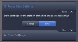
18. Check that the Axioscan can find the focus by pressing 'Auto focus'. Set Fine focussing 'Parameter' to one higher than for the Coarse focussing. Press 'Next'.
